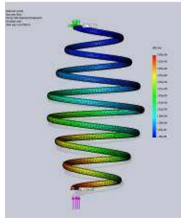
**Figure 11.** Result of displacement
