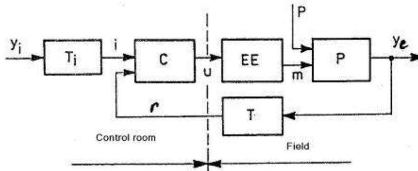
**Figure 1.** Control system of gas pressure regulators
