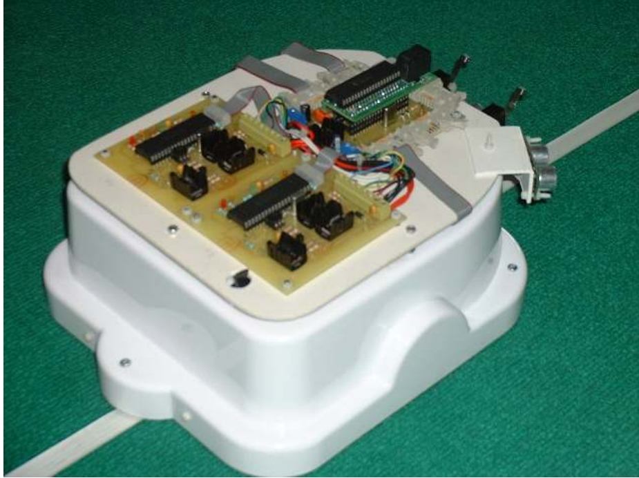
Figure 13. Automatic guided vehicles equipped with microcontroller PIC 16F877
