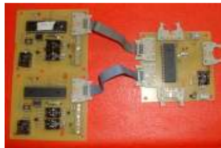
Figure 8. Current regulators and control
