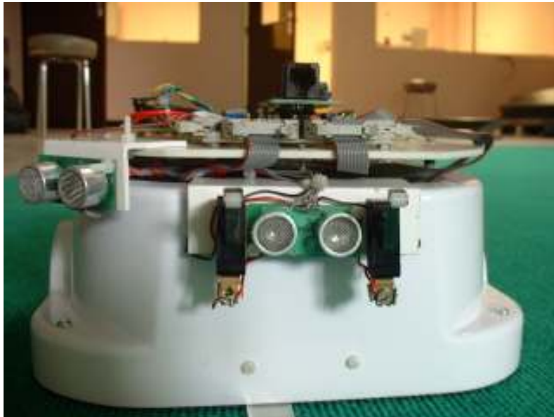
Figure 12. Automatic guided vehicles equipped with microcontroller PIC 16F877
