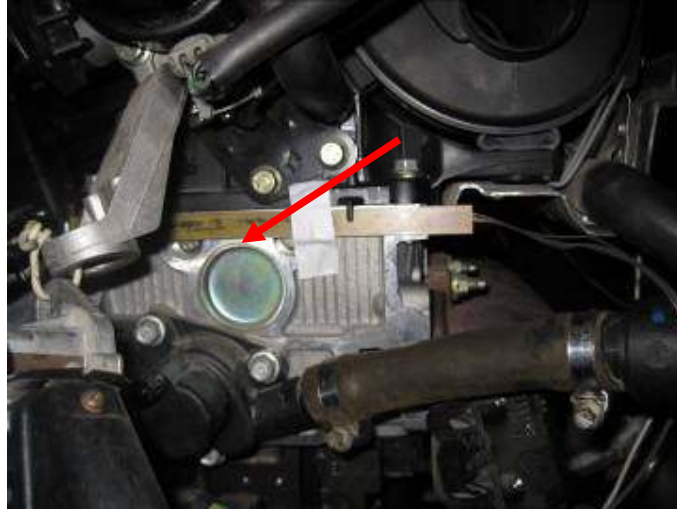
Figure 6. Measurement of temperature with temperature sensor
