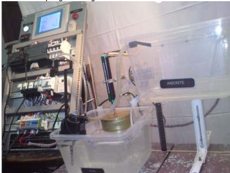
Figure 3. The experimental model for the study of automating a system of pumping water from upstream to downstream hydropower plant using Siemens S7-200 PLC.
