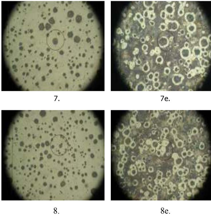
**Figure 1.** Metallographic structure of modified grey cast irons (100X) (e – Nital etched of the sample, 4%)
