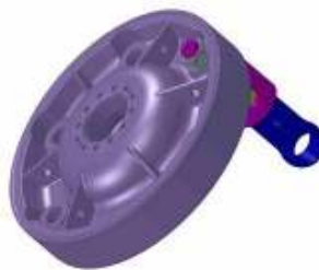
Figure 11. The geometric relationship between the Kaplan turbine fork head and the hexagonal nut M225x4
