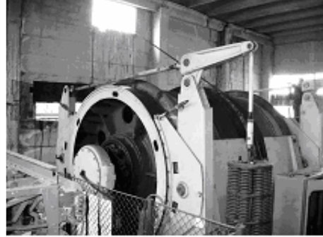
Figure 2. Winding machine Lupeni Mine „No. 12 auxiliary shaft”
