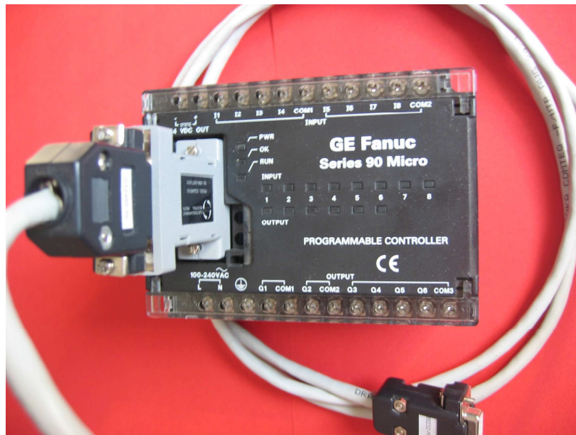
Figure 8. PLC and programmable cable connection to PC
