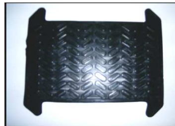
Figure 4. Elastic plate model of PR3 type
