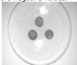
Figure 2 Electrochemically conductibilised plastic material pills (ABS)
