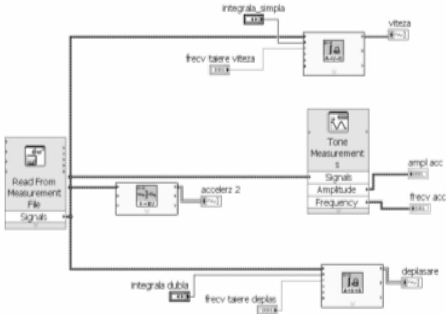
**Figure 2.** The block diagram of the virtual instrument used in reading the dates
