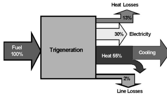
**Figure 1.** Combined heat, cooling and power production
