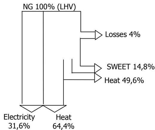
**Figure 3.** Breakdown of energy flow, "winter/CHP" versus "summer/CCHP"
