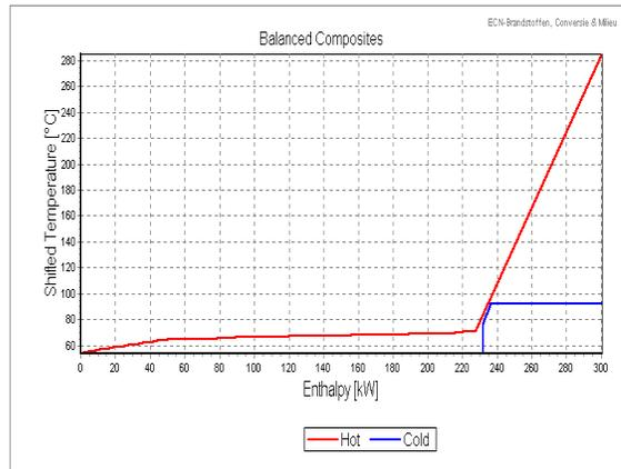
**Figure 2.** Quantity and temperature level of the available heat of a 150 kW<sub>e</sub> CPO-PEMFC cogeneration system, compared to the heat and temperature demand of the SWEAT system.
