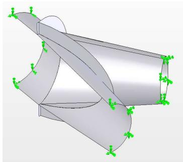
**Figure 3.** The *Fixed* constraints of the branch pipe
