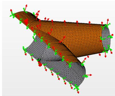
**Figure 6.** The mesh of the branch pipe without ribs
