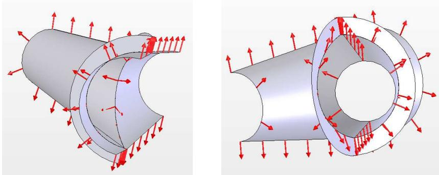
**Figure 5.** Internal pressure applied inside of the piping
