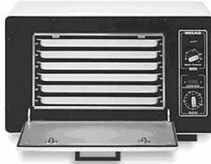
**Figure 1.** Dry heat sterilizers
