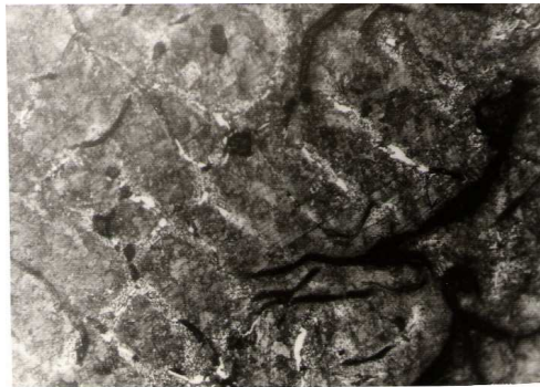
Figure 3. The metallographic structure of the material in the welded area – interior of the sample: the basic material (sample 3) (100X).
