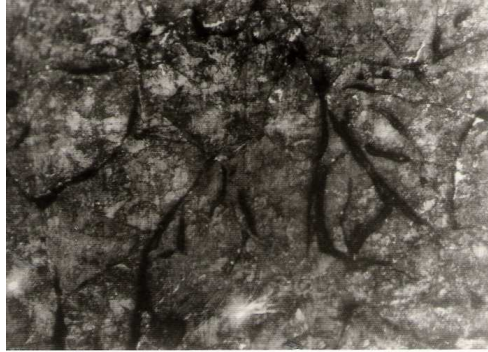
Figure 2. The metallographic structure of the basic material (experimental sample) (Sample 1) (100X).
