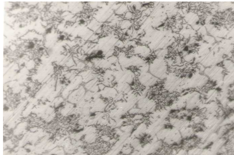
Figure 4. The metallographic structure of the material in the welded area – exterior of the sample: adding material (Sample 4) (100X).
