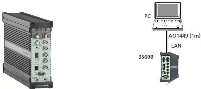
**Figure 6.** Data acquisition front-end: general view and connection to PC
