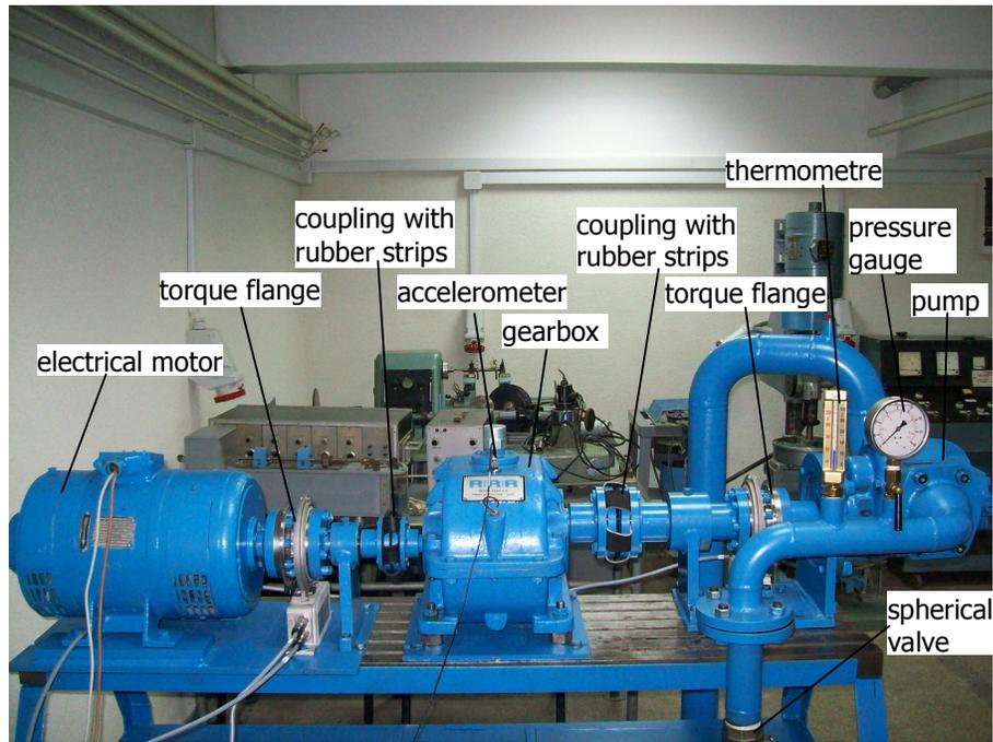
**Figure 3.** General view of the test rig
