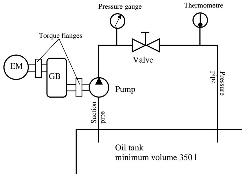
**Figure 2.** Oil flow circuit
