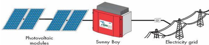
**Figure 1** Principle scheme of a solar photovoltaic system connected to the public grid
