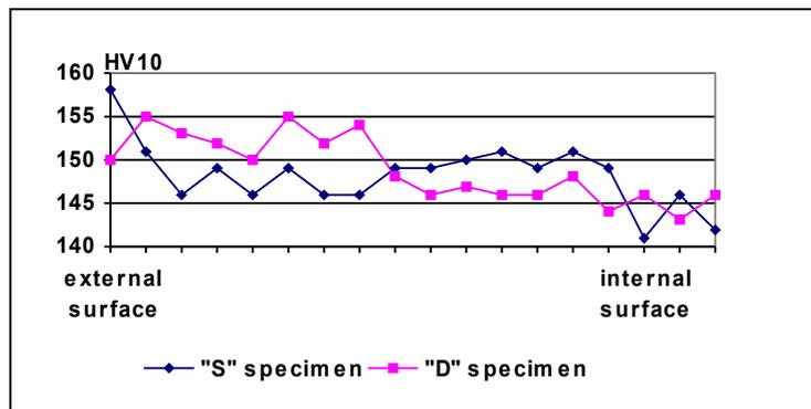
Figure 4. The HV10 hardness values for the "S" and "D" specimens
