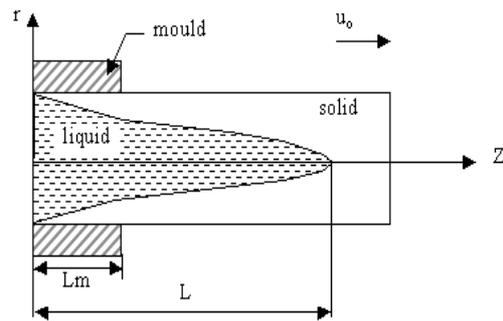
**Figure 3.** r-z coordinates attached to mould
