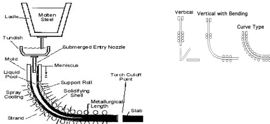
**Figure 1.** Schematic representation of the continuous casting process
