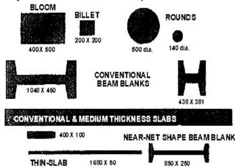
**Figure 2.** Continuously cast sections
