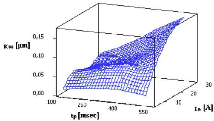
**Figure 11:** Estimated response surface of  $K_w$  variation versus  $I_e$  and  $t_p$
