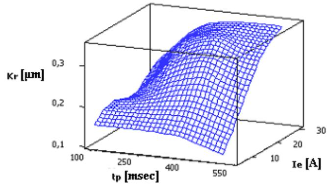
**Figure 10:** Estimated response surface of  $K_r$  variation versus  $I_e$  and  $t_p$
